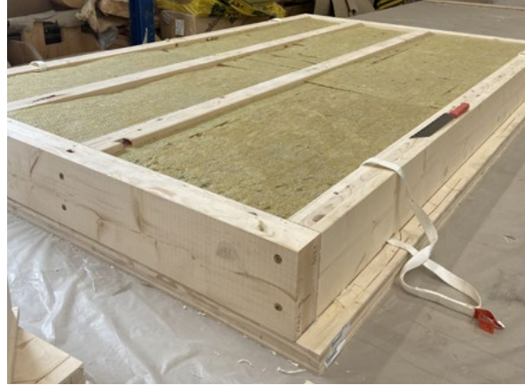
Moulded lifting straps.
