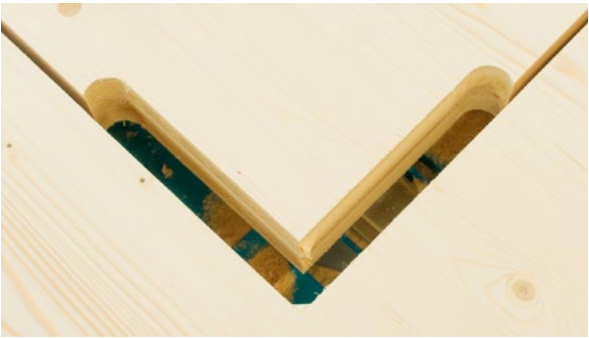
2. Final cutting with a milling cutter – execution with a radius (visual quality).
