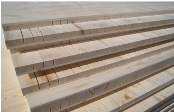
Preparation of connection and installation SOLID 62 mm.
