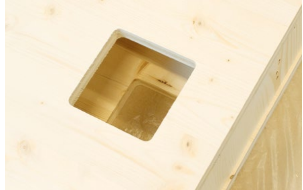
Milling of angular openings, execution with a radius.
