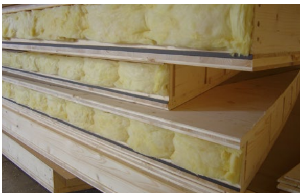
Fitting of insulation into the longitudinal joint.
