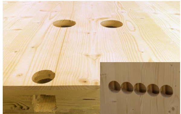
Machining for installations.
