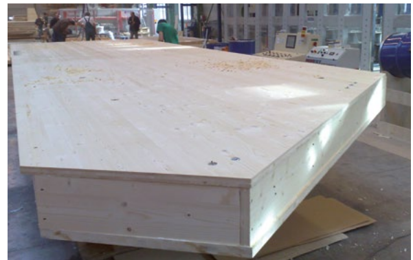
Chamfer cut of the whole element.
