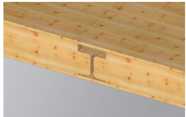
Machining of installation – two-stage.
