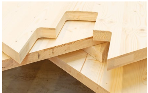
Final cutting of the shape with a shank cutter (with a radius).
