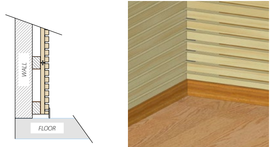
Detail of finishing with a slat
