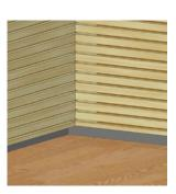
A detail of finishing the acoustic panel 50 mm above the floor
